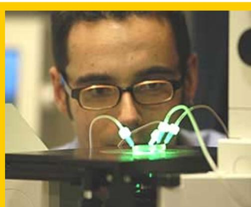
This neon-lit, transparent microfluidic device, seen here on an inverted stage microscope, allows Stoeber to visualize the route particles travel as they enter a small channel, much like the microneedle channels in the chiclet-sized syringe.
