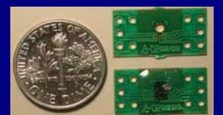
Each ImmunoSensor chip is fabricated using bulk processes similar to the way integrated circuits are manufactured.
