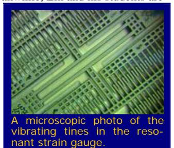
A microscopic photo of the vibrating tines in the resonant strain gauge.
