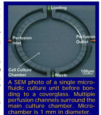
A SEM photo of a single microfluidic culture unit before bonding to a coverglass. Multiple perfusion channels surround the main culture chamber. Micro-chamber is 1 mm in diameter.
