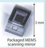
Magnetically Actuated Scanning Micromirror CMOS-compatible actuation voltage (< 3V) High-frequency operation (up to 70kHz) Large scanning angle,  $\leq 80^{\circ}$ , with low power consumption Embedded scanning angle sensor
