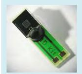
LSCAN Individual Micromirror Module 3-24kHz, 9-18 deg.
