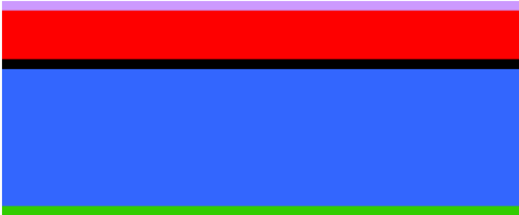
FIGURE 1.3. A phosphosilicate glass layer (PSG) is deposited, and the wafers are annealed at 1050°C for 1 hour in Argon to drive the Phosphorous dopant into the top surface of the Silicon layer. The PSG layer is subsequently removed using wet chemical etching.
