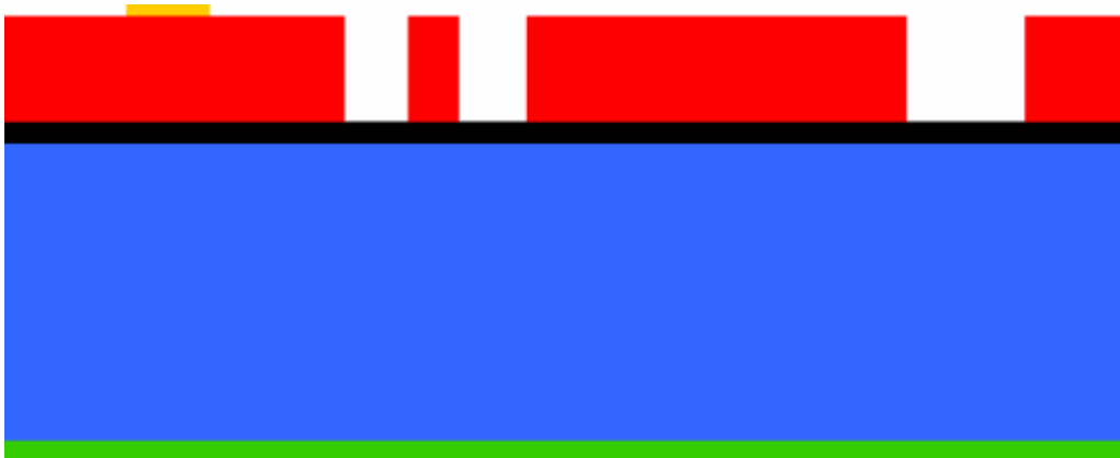
FIGURE 1.5. The wafers are coated with UV-sensitive photoresist and lithographically patterned by exposing the photoresist to UV light through the first level mask (SOI), and then developing it. The photoresist in exposed areas is removed, leaving behind a patterned photoresist mask for etching. Deep reactive ion etching (DRIE) is used etch the Silicon down to the Oxide layer. After etching, the photoresist is chemically stripped.
