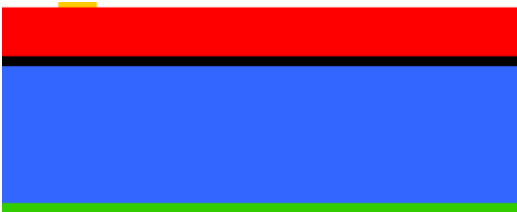
FIGURE 1.4. The wafers are coated with negative photoresist and lithographically patterned by exposing the photoresist with light through the first level mask (PAD METAL), and then developing it. A metal stack consisting of 20 nm chrome and 500 nm gold is deposited over the photoresist pattern by e-beam evaporation. The photoresist is then dissolved to leave behind metal in the opened areas.
