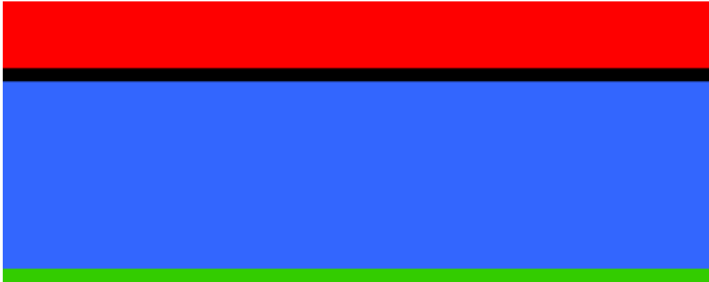
FIGURE 1.2. The SOI wafers consist of a 10µm Silicon layer, a 1µm Oxide layer, and a 400µm Substrate layer. A Bottom Side Oxide layer is also initially present on the wafers.
