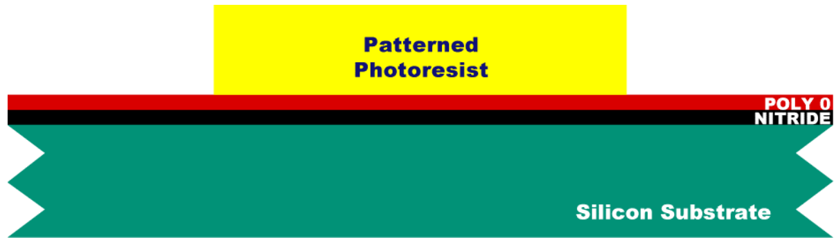
Figure 1.3. The photoresist is lithographically patterned by exposing it to UV light through the first level mask (POLY0) and then developing it. The photoresist in exposed areas is removed leaving behind a patterned photoresist mask for etching.
