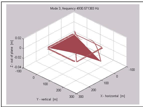
Fig.2 Mode 3 of a modal analysis of parallel plate accelerometer rotator using the plate and beam elements, the figure displays the plate using the display functions developed for plates.
