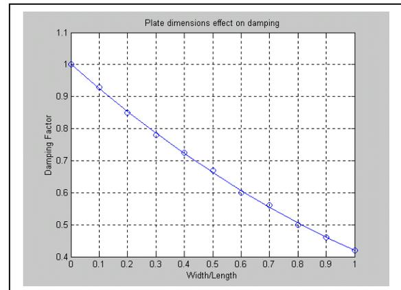
Fig.3 Effect of width/Length ratio on Damping produced by a rectangular plate.
