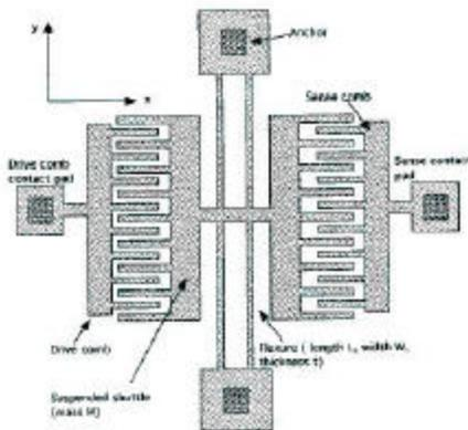
**Fig. 4. Electrostatic comb-drives**
