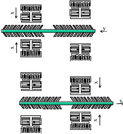
**Fig. 3. Two-step operation of the linear micro-motor**
