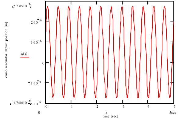
**Fig. 5.** simulation plot of displacement vs. time at resonant frequency  $w_n = 7.4\text{kHz}$  with  $t=L=g=2\text{mm}$ ,  $N_g=50$ ,  $V_{dc}=50\text{V}$ ,  $v_{ac}=12\text{V}$ .
