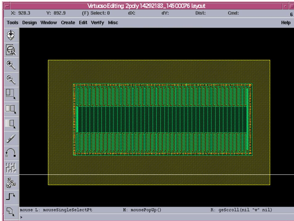
**Fig. 3 electrostatic comb-drive**
