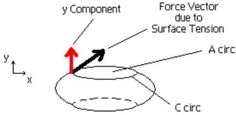
**Figure 3b:** Model of force due to surface tension in an air bubble.
