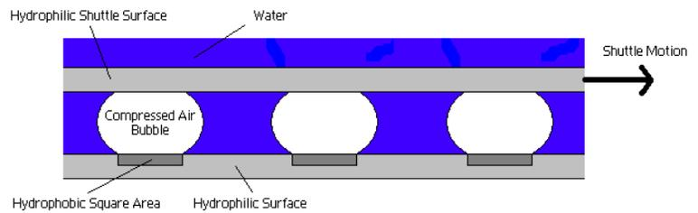
**Figure 2b:** Schematic of hydrophilic polysilicon shuttle riding on air bubble array.
