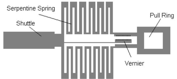
**Figure 2a:** Schematic of serpentine force gauge with integrated hydrophilic shuttle.
