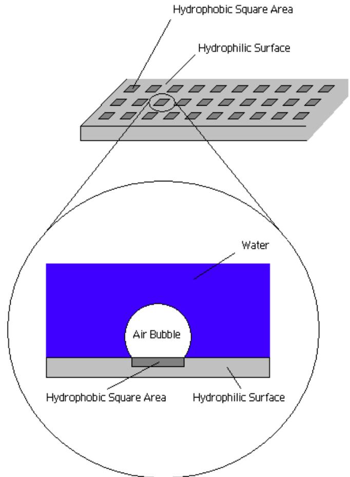
**Figure 1:** Schematic of hydrophobic-hydrophilic patterned substrate with resulting air bubble formation.
