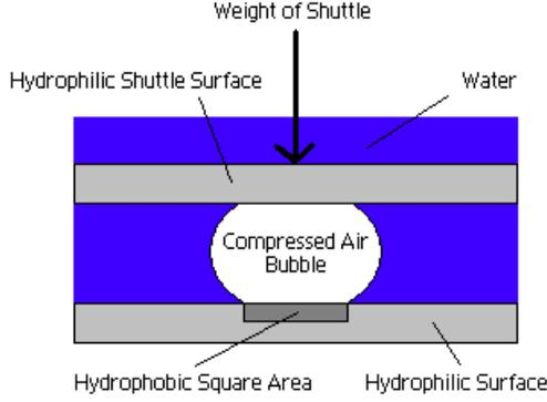
**Figure 3a:** Theoretical model of air bubble subjected to hydrostatic pressure and uniaxial compressive loading.
