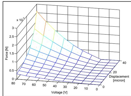
**Figure 4:** Theoretical force exerted by MIPARF versus applied voltage for different nodal displacements
