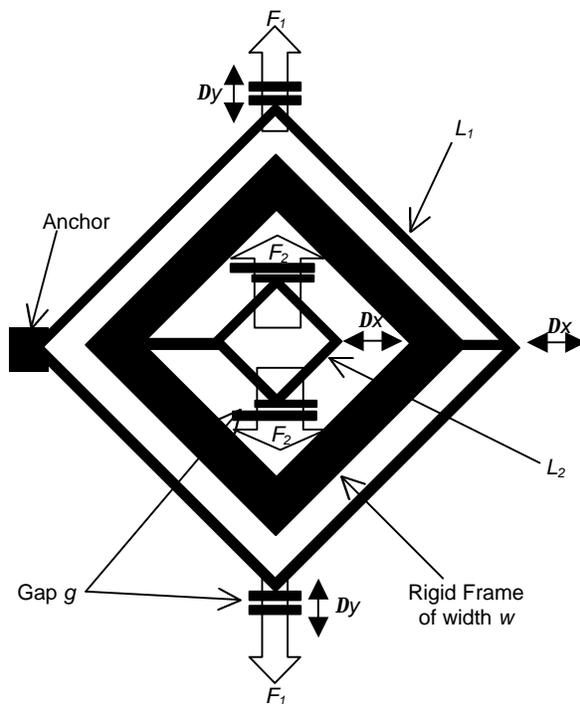
**Figure1:** Principle behind the motion and transformation of the multiple inter-connected parallelogram actuators and rigid frames
