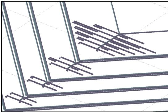
**Figure 3:** For the inner actuators, the path of the beam connecting the gap-closers to the parallelogram structure should be clear of the anchored electrodes while the overlap area should remain constant throughout the actuation.
