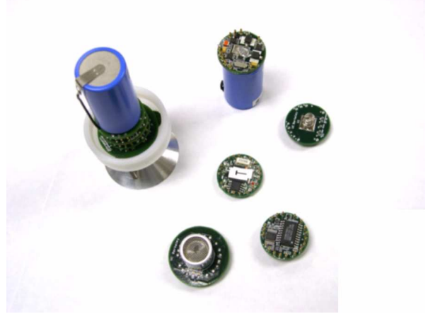
Figure 3: Our experimental hardware consists of Mica2Dot motes (center), and clockwise from the top: rechargeable battery with top-mounted power adapter board, recharger contact board, HoneyDot magnetometer (unused in this experiment), ultrasonic transceiver board, and the complete sensor node including an inverted cone for reflecting the ultrasonic signal omnidirectionally.
